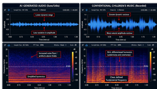
Figure 4. Waveform and spectrogram comparison between an AI-generated children’s song sample and a conventional recorded children’s song.
