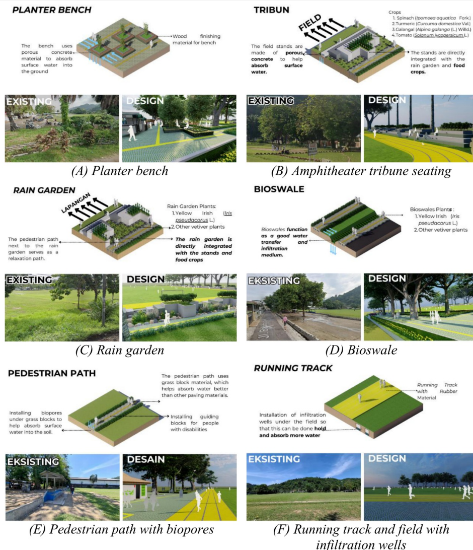
Figure 11. Integrated modular components of the urban agriculture-based floodable park: (a) planter bench, (b) amphitheater tribune seating, (c) rain garden, (d) bioswale, (e) pedestrian path with biopores, (f) running track and field with infiltration wells.
